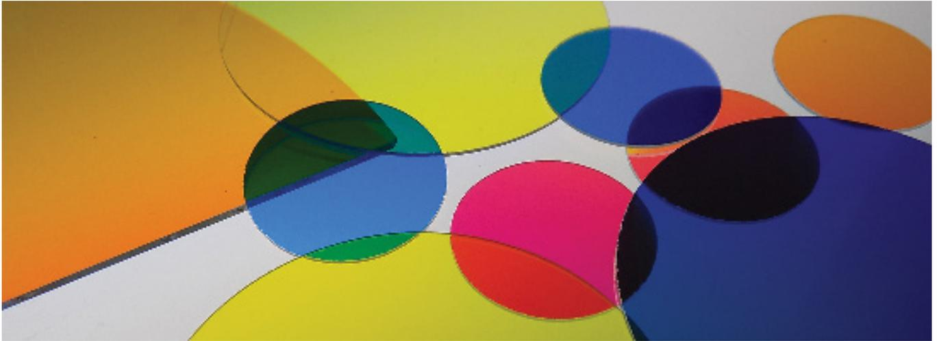
Dichroic filters, widely used in the lighting industry, are composed of a substrate generally of borosilicate glass, on which a dielectric coating is deposited, i.e. an alternation of very thin layers of dielectric materials such as silicon oxide and titanium, with different refraction indices.
